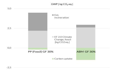
Figure 3: GWP for two GFRP materials, a fossil- and a bio-based ABM alternative (Environmental footprint v2 database, GaBi)
