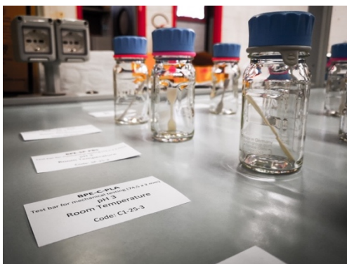
Figure 2: Samples being prepared for Water Uptake testing.
