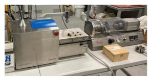
Image 2: Device for the production of sample specimens: mini extruder & injection molding machine for production of test specimen for toys and baits (Source: ACIB).
