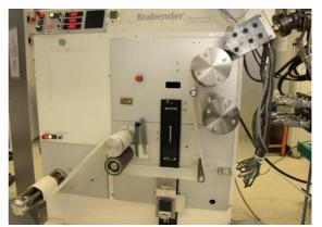
Image 3: Production of samples: bio-based plastic film being calendered, a process in which the polymer melt is stretched, cooled and collected to a film of desired thickness using a series of rollers (Source: Fraunhofer LBF).
