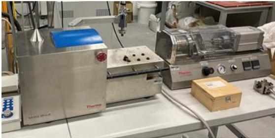
*Image 2: Device for the production of sample specimens: mini extruder & injection molding machine for production of test specimen for toys and baits (Source: ACIB).*
