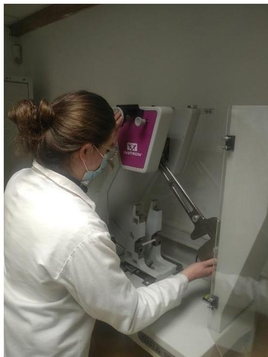
*Image 5: Charpy impact test on a test bar (Source: NaturePlast).*
