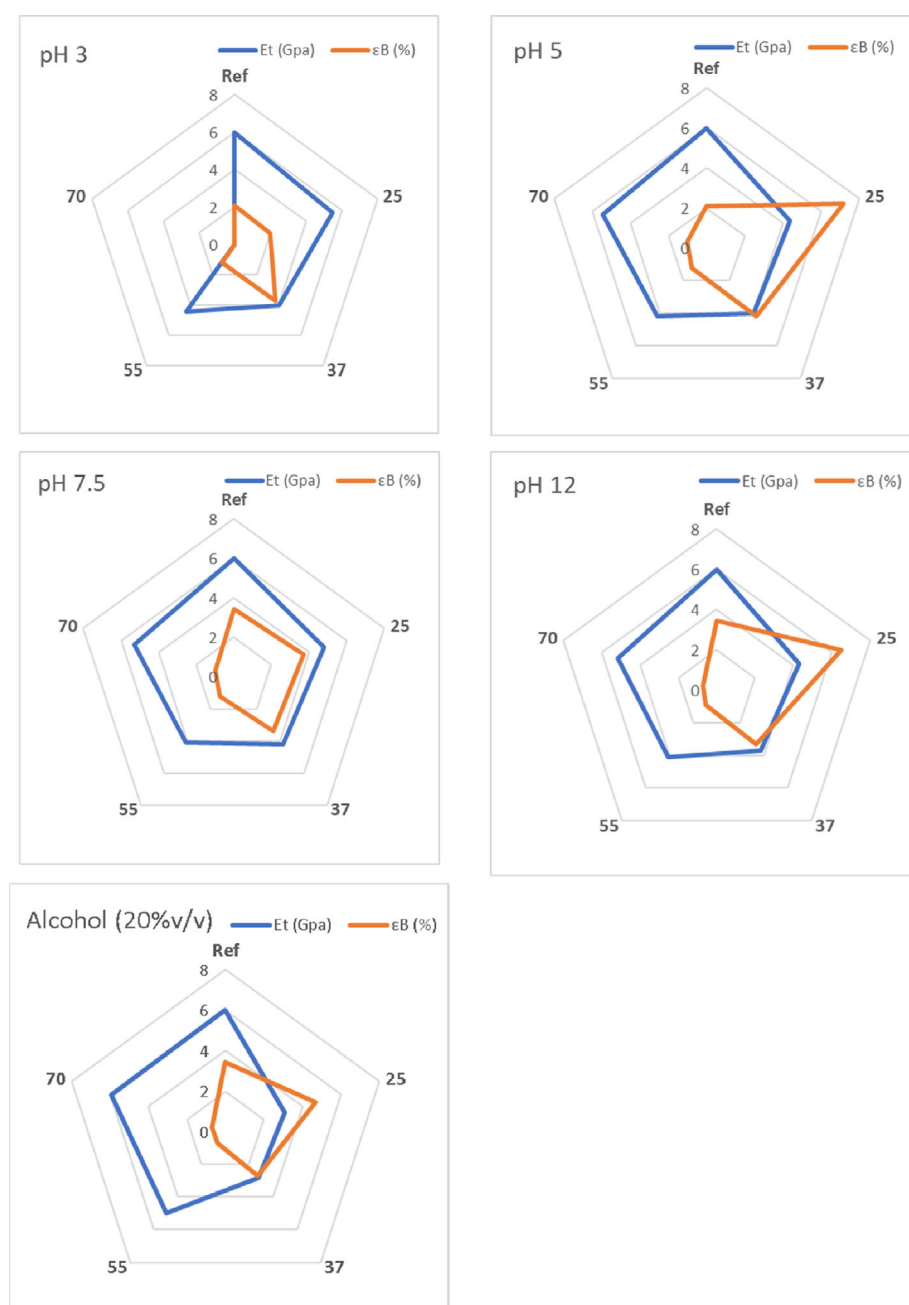
FIGURE 4 Radar charts representing the tensile Young's modulus ( E_t ) and the strain at break ( \epsilon_B ) at the different testing temperatures and immersion media. [Color figure can be viewed at wileyonlinelibrary.com ]
